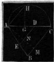
$$AD^2 : AC^2 = q : Q \text{ и } AD = AC \cdot \sqrt{\frac{q}{Q}}. \text{ При } Q = 6300 \text{ к. с. и } q = 1008 \text{ к. с. будетъ } \frac{q}{Q} = \frac{1008}{6300} = \frac{112}{700} =$$
